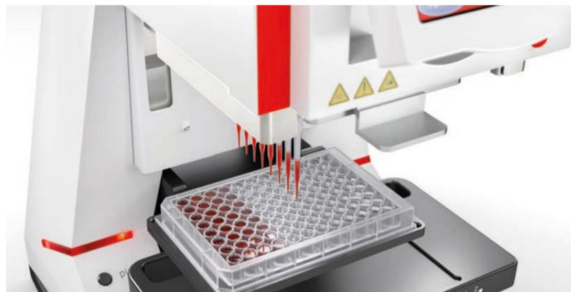
Serial dilution is very simple using the 8 channel magazine in combination with the serial dilution pipetting mode.
