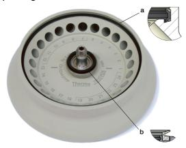
Top detail: Large seal in outer groove of rotor body; bottom detail: small seal in groove of rotor collar
