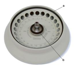
a = Large seal in outer groove of rotor body; b = Small seal in groove of rotor collar Figure 5: Rotor Lid Seals
