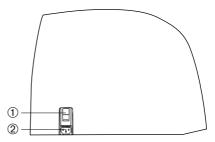
① Power Supply Switch; ② Mains Connection
